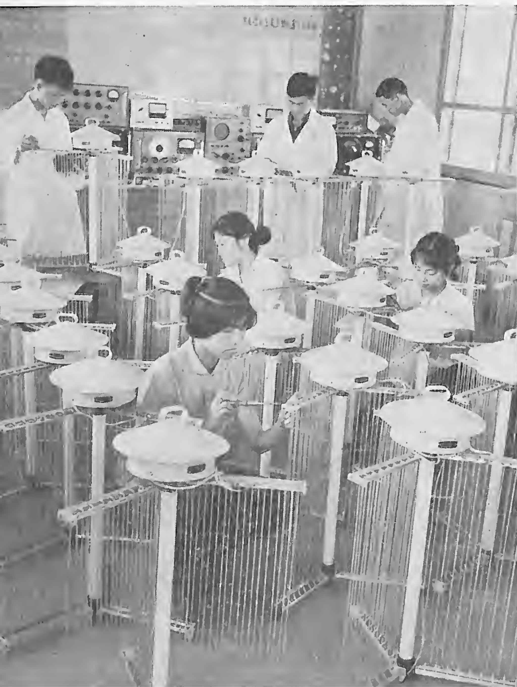
The Fengshun County Radio Plant in Kwangtung province makes low-voltage transistorized D-C ultra-violet lights for field use in insect extermination.
